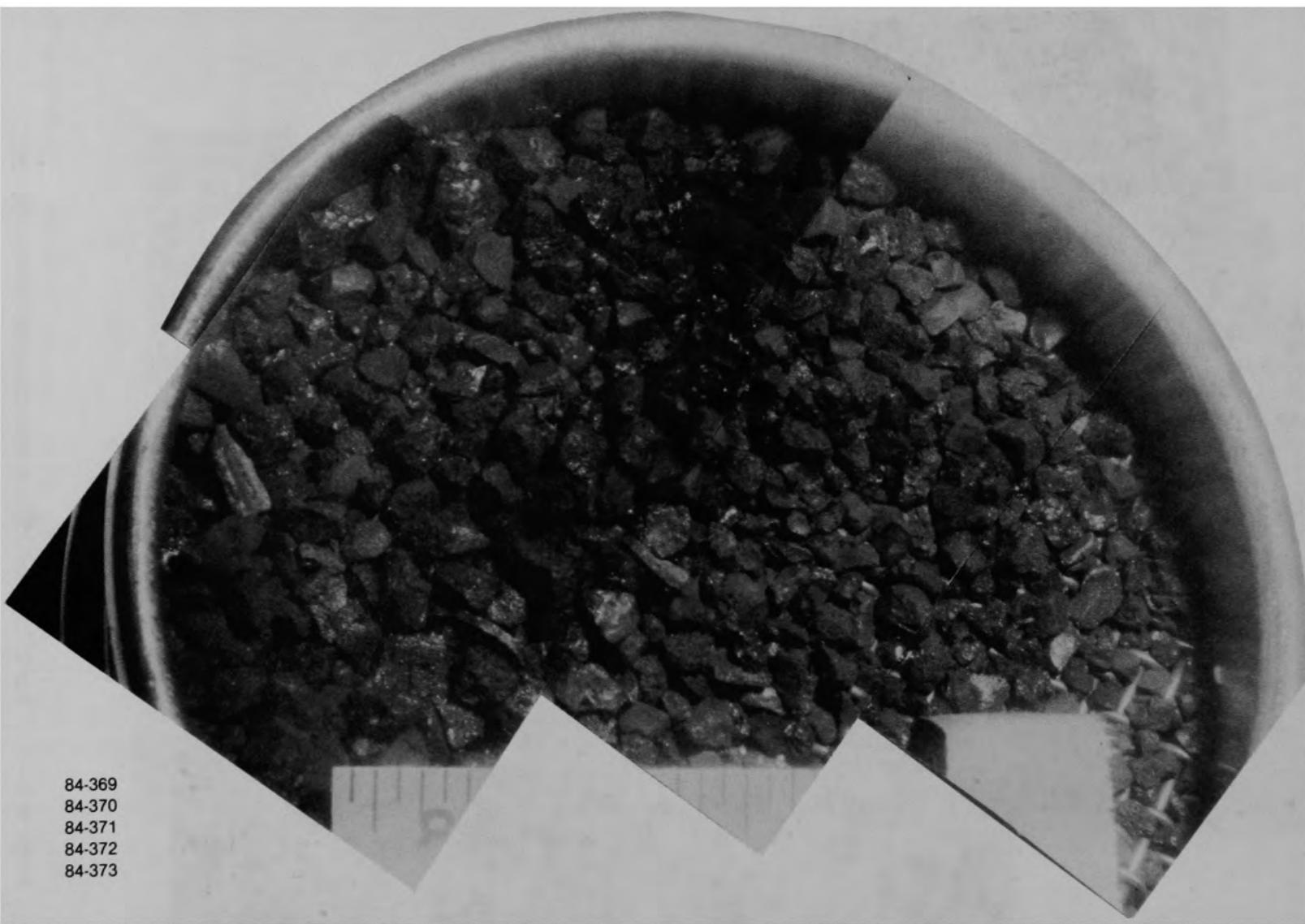
Figure B-45. Particle size fraction (size range: 1680-4000  $\mu\text{m}$ ) from Sample 8, (H8, 70 cm).
